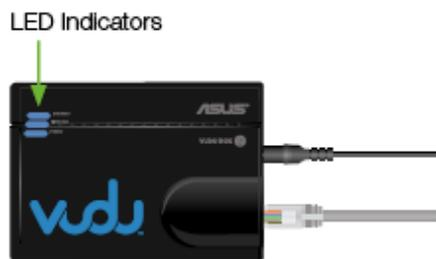
Going forward, all three LED indicators on both wireless adapters should be illuminated. When the LED indicators for Wireless and Ethernet start to blink, data is being transmitted.
