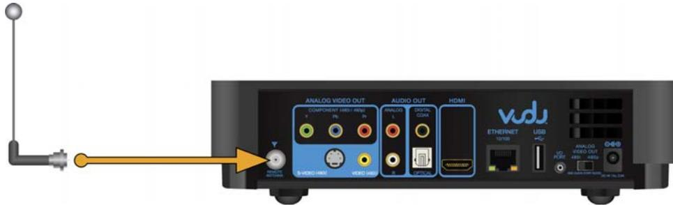
*Note: The VUDU remote is a radio frequency, or RF, remote. This means you don't have to point it at the VUDU Internet Movie Player for it to work. Because RF remotes use radio waves, however, it is imperative to use the antenna in order for the player to receive input from the remote.*
