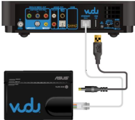
3: Place the VUDU Internet Movie Player where you plan to keep it. Then, connect the player to a power source using the enclosed power supply and AC cord. (First connect the cord to the player and then plug it into the outlet.)
