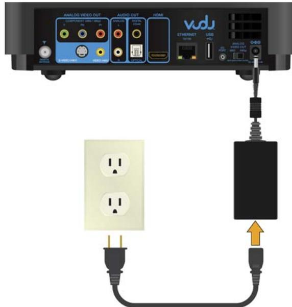
**Warning:** Do not move the VUDU Internet Movie Player while it is plugged into a power source. This may cause significant damage to the hard drive, resulting in loss of data or functionality.
